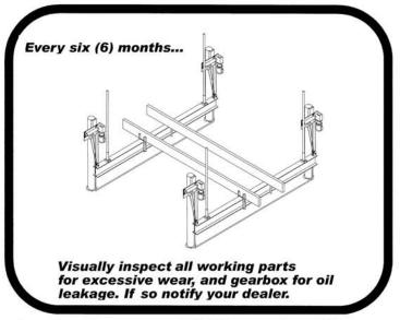
MAINTENANCE TIP: To keep your Hi-Tide lift operating at peak performance, minimizing service calls, we recommend that you operate your lift occasionally during the off-season or extended periods of no boating activity. Simply run the lift for approximately one minute in each direction. This will keep the motor contacts and brushes clean and all pulleys and bearings evenly lubricated.
