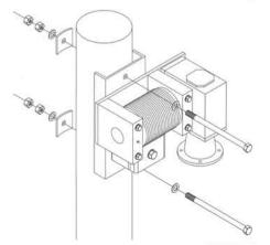
Notch or shim drive unit to insure drive units are level, plumb, and square, then tighten all bolts.
