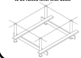
Pre-drill pilings with supplied hole pattern. Top hole should be a min. of 6" from top piling to prevent splitting.
