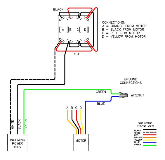
MAIN DISCONNECT AND BRANCH CIRCUIT PROTECTION SUPPLIED BY OTHERS ACCORDING TO CHART BELOW. USE UL489 BREAKER.
