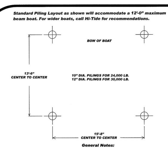
Lifter beams are designed to lift on the side of support pilings, if dock edge overlaps any part of pilings, notch deck boards to accommodate lifter beams. The depth of water required is approximately 24" plus the hull draft of the watercraft. It is the contractor's responsibility to determine and construct suitable support fixtures and bracings for lift pilings. Call Hi-Tide as needed.
