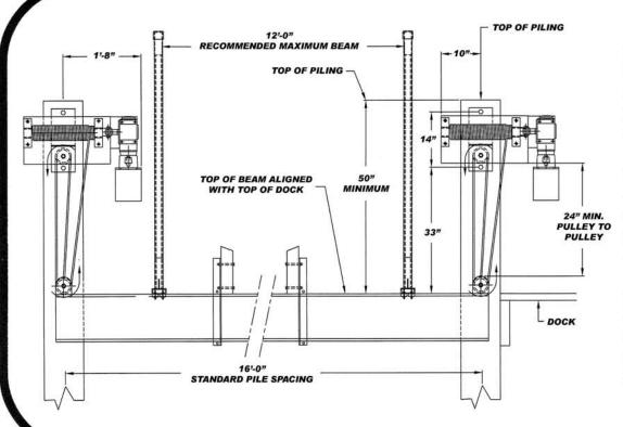
Must have a min. 50" of piling above highest point of travel of the cradle beam.
