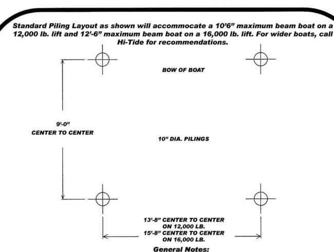
Lifter beams are designed to lift on the side of support pilings, if dock edge overlaps any part of pilings, notch deck boards to accommodate lifter beams. The depth of water required is approximately 18" plus the hull draft of the watercraft. It is the contractor's responsibility to determine and construct suitable support fixtures and bracings for lift pilings. Call Hi-Tide as needed.
