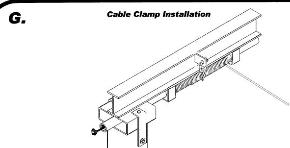
Insert cable into winder hole and push until cable emerges from end of pipe. Attach cable clamp and pull cable back until clamp rests against the backside of the winder hole. Lift cables should be adjusted such that the boat sits on the cradle at the same attitude as the boat sits in the water to assure good rain drainage. For typical installation, shorten bow cables as follows: 4,000 Lb. – 6,000 Lb. = Approx. 2", 9,000 Lb. – 16,000 Lb. = Approx. 4"
